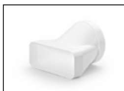
9700 537 Rectangular/round adapter: Section 227x94 mm / ø 158 mm dim: 190x 150x227 mm
